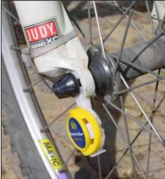
The timing chip will be attached to a front fork mount. Remove the front wheel quick release and attach the chip mount as shown to your front wheel skewer.
